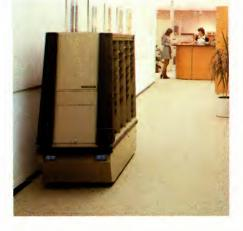
The unit moves at a safe speed of only about one mile an hour (1.5 feet per second); slower than the average person walks. An audible soft tone and pair of flashing blue lights add to its safe operation.
